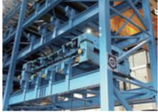
Loading and unloading station of 40,000-ton press
