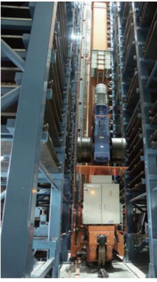
AS / RS for 20,000-ton press machine molds
