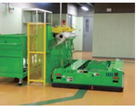
Paper tube collection machine and accumulating machine
