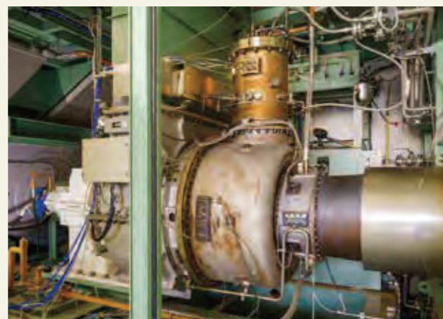
2,000-kilowatt-class gas turbine co-firing liquid ammonia and natural gas at IHI Yokohama Works
